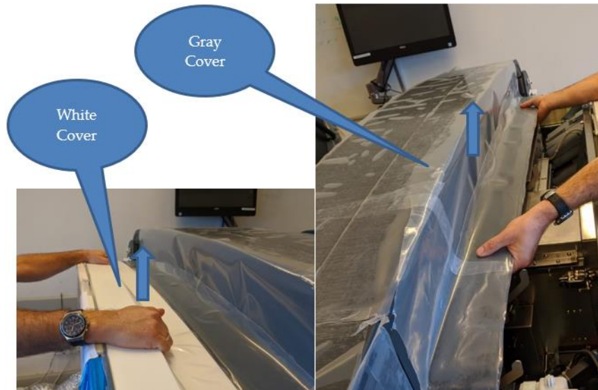
Figure 86 Opening covers to replace feeding wheels
