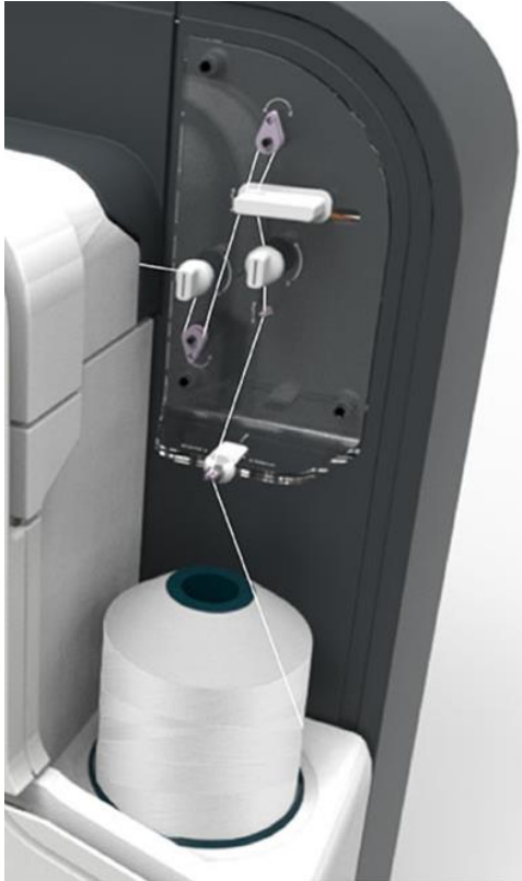
Figure 30 Completed thread guiding path
