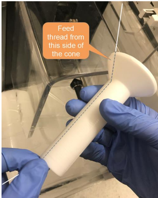
Figure 32 Feeding the thread through the large end of the cone
