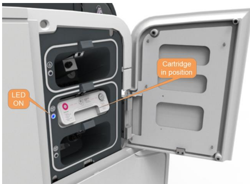
Figure 19 Empty waste cartridge inserted. Blue LED is ON.
