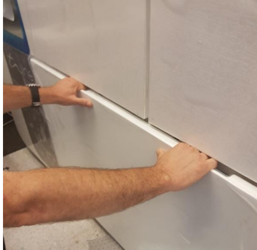
Figure 92 Opening the lower front cover
