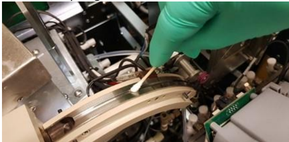
Figure 88 Cleaning the dyeing head
