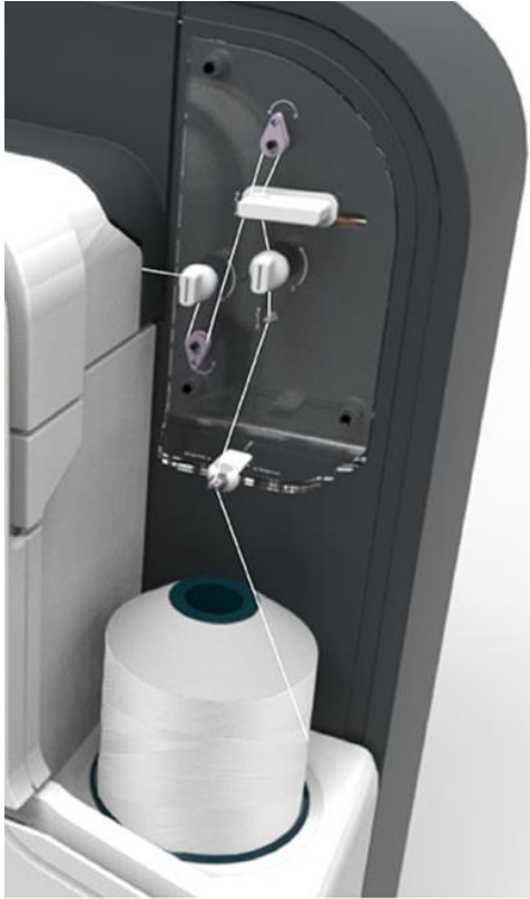
Figure 28 Completed thread guiding path
