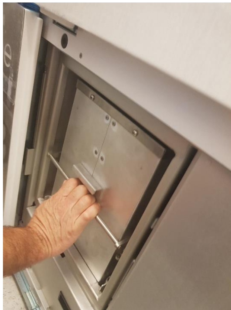
Figure 95 Installing the carbon filter
