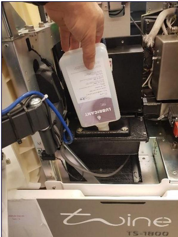
Figure 28: Filling the lubricant
