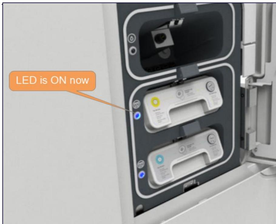
Figure 23: Empty waste cartridge inserted
