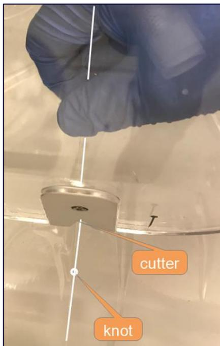
Figure 55: Cutting the thread at the winder
