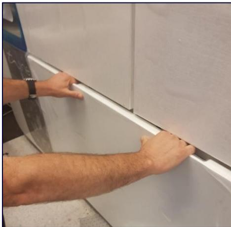
Figure 122 Opening the lower front cover
