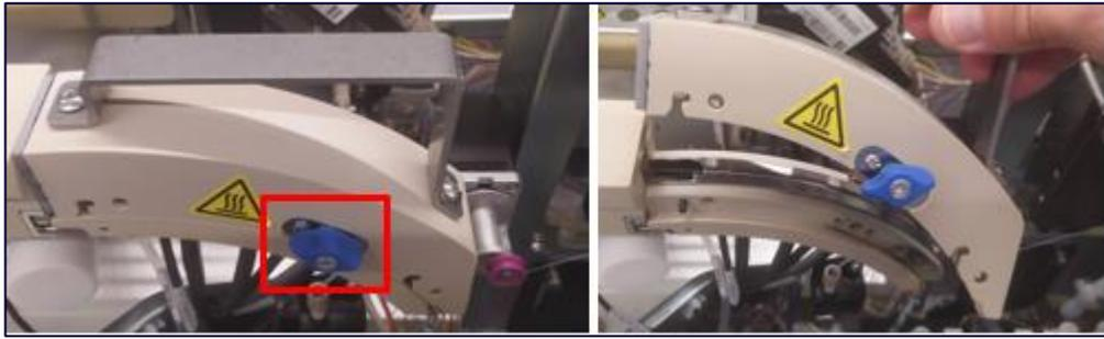
Figure 37: Open the Arc cover lock screw
