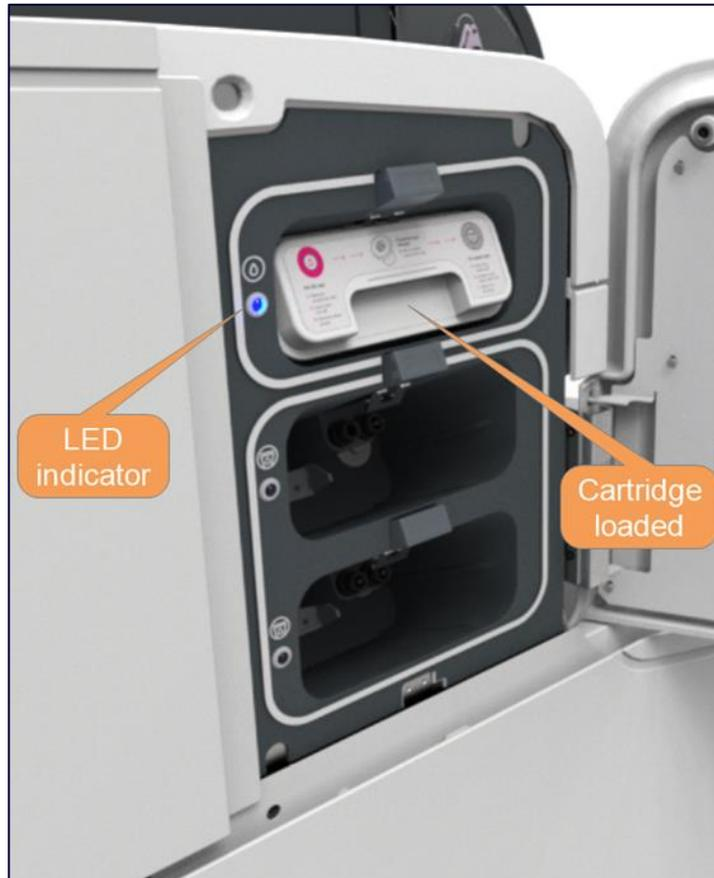
**Figure 11: Ink cartridge loaded**
