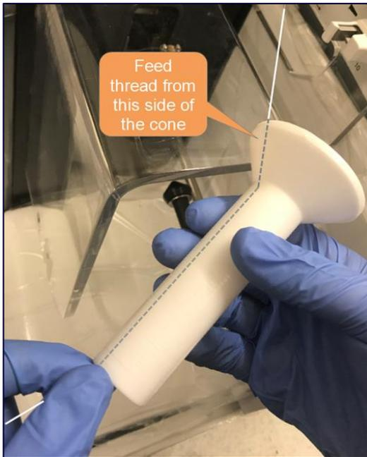
**Figure 44: Feeding the thread through the wide end of the cone**
