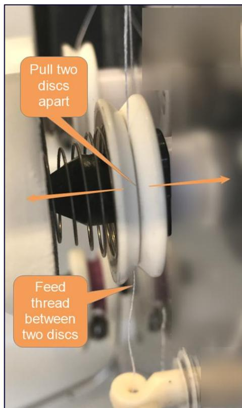
Figure 33: Feed the first guide lock
