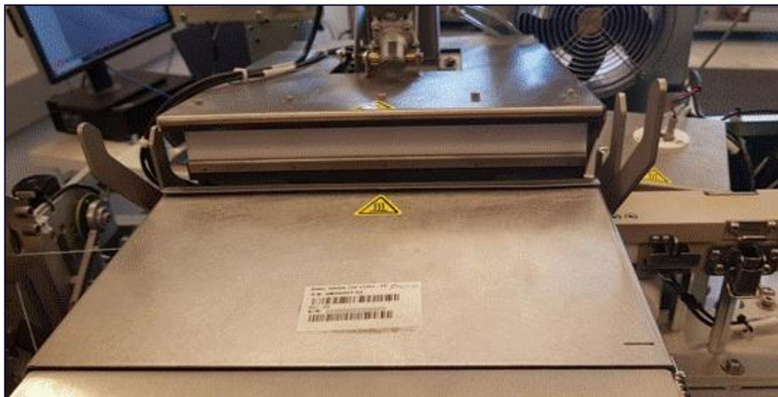
**Figure 39: Open upper door of dryer**
