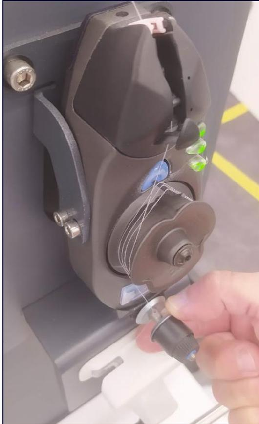
Figure 35: Feed the Thread through the B TSR tensioner and B TSR wheel
