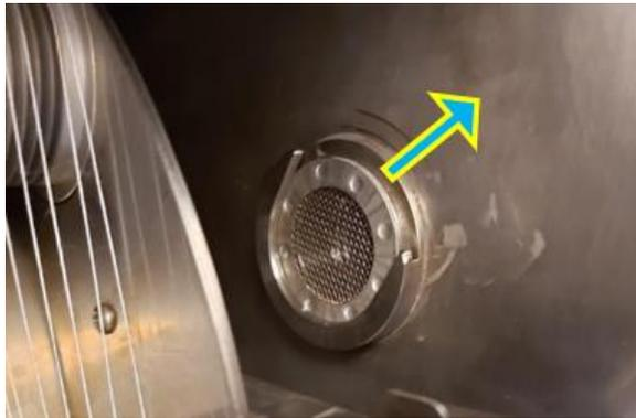
Figure 114: Pulling out the ring filter
