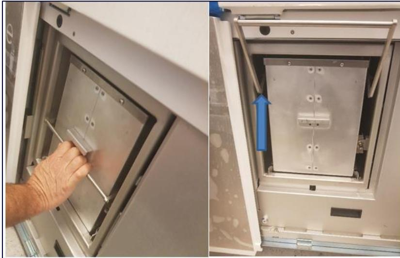
Figure 124: Filter handle raised
