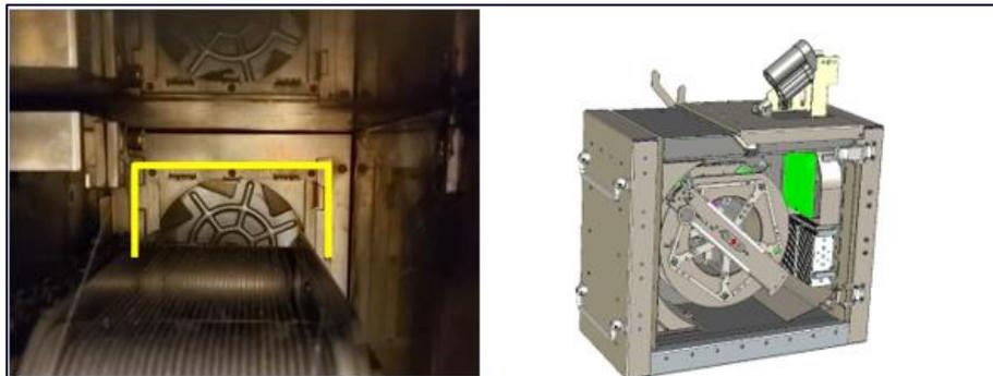
Figure 115: Dryer Rear Filter
