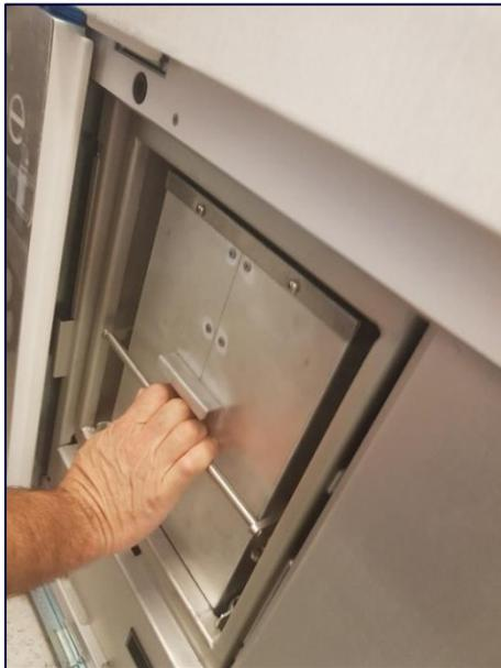
**Figure 127: Installing the carbon filter**
