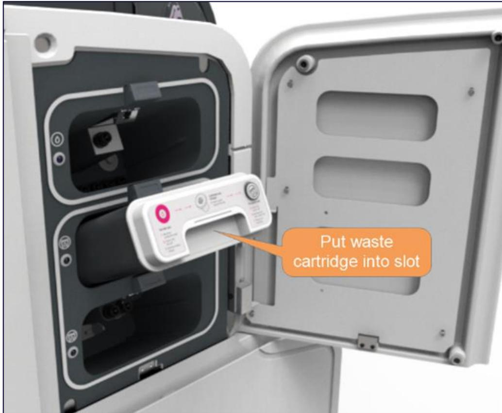
Figure 18: Slide waste cartridge into slot
